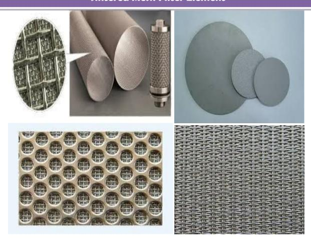
Sintered wire mesh laminates range from single, double to multilayer laminate of fine filter mesh providing a heavy plate or brick like structures consisting of several hundreds of different mesh layers with total thickness up to 2 inch or more. By combining the single mesh layer of numerous weaves, it is feasible to construct materials with a net desired thickness, permeability, pore size and durability.
