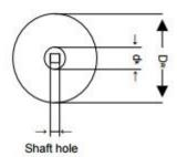
The formula for calculating the roll diameter is  $D_m = 1.27.d.L + d_k^2$
